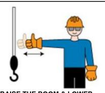
RAISE THE BOOM & LOWER THE LOAD - With arm extended horizontally to the side and thumb point up, fingers open and closed while load movement is desired.
