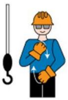
CRAWLER CRANE TRAVEL, BOTH TRACKS - Rotate fists around each other in front of body; direction of rotation away from body indicated travel forward; rotation towards body indicates travel backward.
