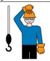
**USE MAIN HOIST -** A hand taps on top of the head. Then regular signal is given to indicate desired action.
