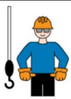
**RETRACTING TELESCOPING BOOM** - with hands to the front at waist level, thumbs point at each othe with other fingers closed.
