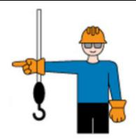
**SWING** - With arm extended horizontally, index finger points in direction that the boom is to swing.
