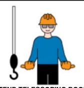
**EXTEND TELESCOPING BOOM** - With hands to the front at waist level, thumbs point outward with other fingers closed.
