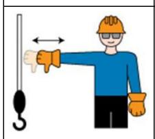
LOWER THE BOOM & RAISE THE LOAD - With arm extended horizontally to the side and thumb pointing dow, fingers open and close while load movement is desired.
