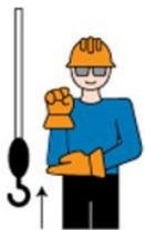
**USE AUXILLARY HOIST** (whipline) - With arm bent at elbow and forearm vertical, elbow is tapped with other hand. Then regular signal is used to indicate desired action.
