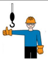
**RAISE BOOM -** With arm extended horizontally to the side, thumb points up with other fingers closed.
