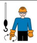
**LOWER -** With arm and index finger pointing down, hand and finger make small circles.
