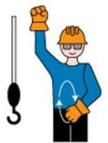
CRAWLER CRANE TRAVEL, ONE TRACK - Indicate track to be locked by raising fist on that side. Rotate other fist in front of body in direction that other track is to travel.
