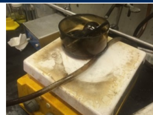
Photo 1. Oil bath that burned.
