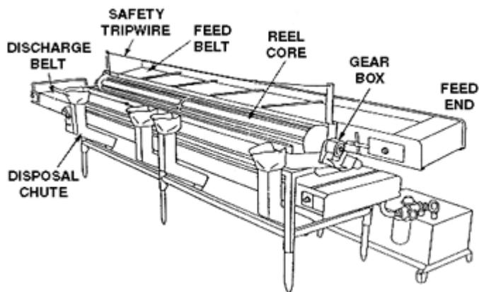
A safety tripwire cable is a device located around the perimeter of or near the danger area. Operator must be able to reach the cable to stop the machine. Tripwire cables must be manually reset to restart the machine.
