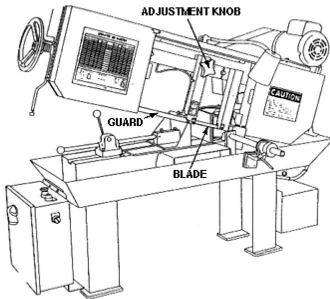
An adjustable guard provides a barrier that may be adjusted to facilitate a variety of production operations. Adjustable guards are useful because they allow flexibility in accommodating various sizes of stock, but, because they require adjusting, they are subject to human error.
