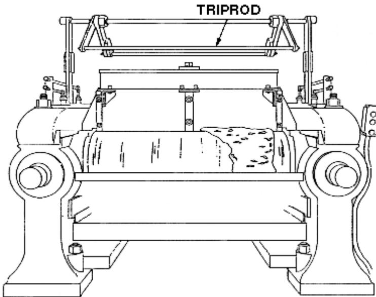
When pressed by the operator's hand, a safety tripod deactivates the machine. Because it has to be actuated by the operator during emergency situations, proper position is critical.
