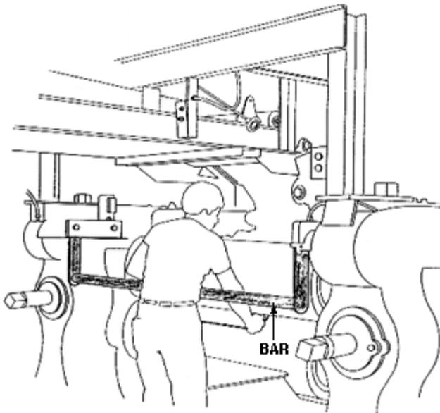
When depressed, a pressure-sensitive body bar will deactivate the machine. If the operator or anyone trips, loses balance, or is drawn into the machine, applying pressure to the bar will stop the operation.
