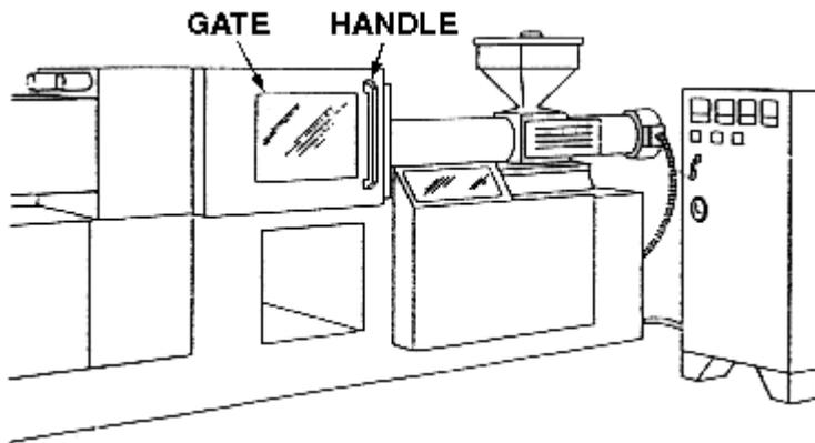
Gates are movable barriers that protect the operator at the point of operation before the machine cycle can be started. Gates are, in many instances, designed to be operated with each machine cycle. If the gate does not fully close, machine will not function.
