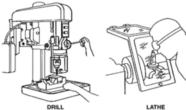
Aids such as clear protective shields do not give complete protection from machine hazards, but do provide some protection from flying particles, splashing cutting oils, and coolants. They provide the operator with an extra margin of safety.
