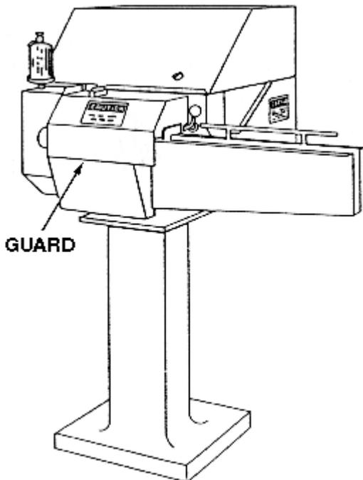
When an interlocked guard is opened or removed, the tripping mechanism or power automatically shuts off or disengages, and the machine cannot cycle or be started until the guard is back in place.
