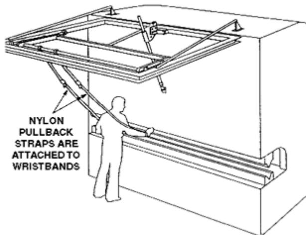
A pullback utilizes a series of cables attached to the operator's hands, wrists, or arms which withdraws hands when the slide/ram begins to descend. It is primarily used on machines with full-revolution stroking action and allows access to the point of operation when the slide/ram is up.
