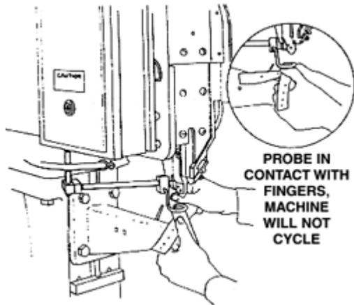
An electromechanical presence-sensing device has a probe or contact bar that descends to a predetermined distance when the operator initiates the machine cycle. If there is an obstruction preventing it from descending its full pre-determined distance, the control unit does not actuate the machine cycle.
