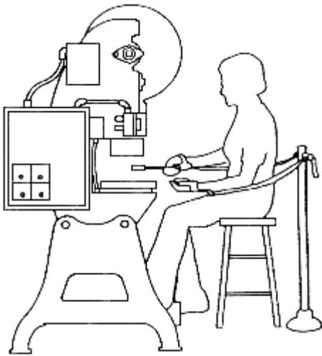
A restraint uses cables or straps attached to the operator's hands and a fixed point. It must be adjusted to let the operator's hands travel within a predetermined safe area.
