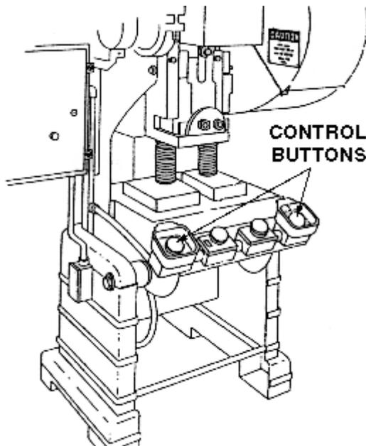
A two-hand control requires constant, concurrent pressure to activate the machine. This kind of control requires a part-revolution clutch, brake, and a brake monitor if used on a power press. The operator's hands are required to be at a safe location (on control buttons) and at a safe distance from the danger area while the machine completes its closing cycle.
