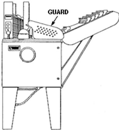
A fixed guard provides a barrier, a permanent part of the machine, preferable to all other types of guards.
