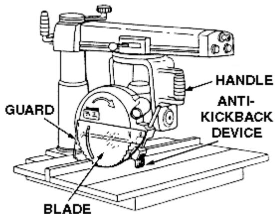
A self-adjusting guard provides a barrier that moves according to the size of the stock entering the danger area. Self-adjusting guards avoid the potential for human error associated with adjustable guards.
