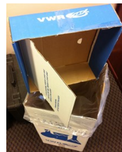
Figure 3. White panel of lid stays pointing downward on the exterior of the liner and bottom half of container until it is filled.
