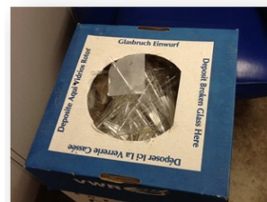
Figure 1. Container which is missing a liner and overfilled; preventing the lid from being shut and secured.
