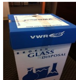
Figure 5. Building services employees have been instructed not to dispose of a broken glass container unless it is intact, lid in place, and taped shut.
